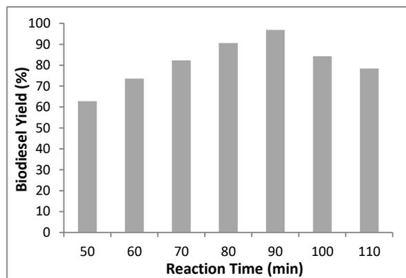
**Fig. 5.** Variation of WCOB yield with the change of reaction time while other parameters were kept constant (temp.: 60 °C, methanol: 50 wt.% and NaOH: 0.8 wt.%)
