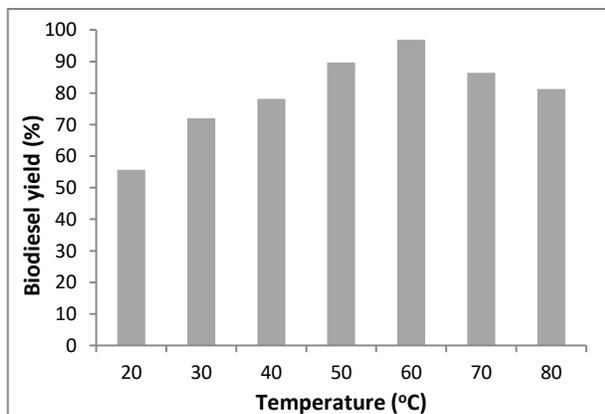
**Fig. 4.** Variation of biodiesel yield with the change of temperature while other parameters were kept constant (time: 90 min, methanol: 50 wt. % and NaOH: 0.8 wt.%)
